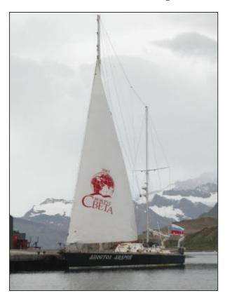
The "Apostol Andrey" is a Russian oceanic yacht launched in 1996. She has a steel hull, is 16.2 metres long and 25 tons. She is Bermuda Ketch rigged and normally carries a crew of 6.
