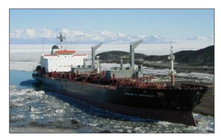
For the 1999-2000 Austral summer season the United States Antarctic Programme used the Military Sealift Command common user tanker "Richard G. Matthiesen" for its supply run to McMurdo Sound. The vessel is 39,624 tons displacement and was particularly suited to this task as it has a double hull and is also ice strengthened. It was built in 1985 and has hull number T-AOT 1124.
