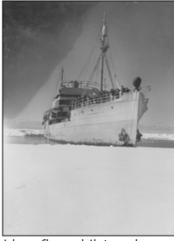
The R.R.S. Discovery II stopped alongside a floe whilst and anchor is taken inboard to prevent it becomming foul of ice (1935)
