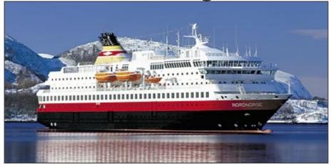
The "Nordnorge" was built in 1997 for the Norwegian Coastal Fleet and during the northern summer operates between Bergen and Kirkenes. She was built to navigate shallow and narrow waters as well as open sea and is classified for light ice conditions. She normally carries 460 passengers but during Antarctic operations this will be limited to 350 passengers. The "Nordnorge" uses eight zodiacs while in the antarctic and is restricted by I.A.A.T.O. to having 100 passengers go ashore at any one time.
