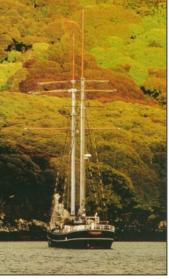
The "tradewind" is a 2 masted historic sailing vessel which in the late 1980's was based in the South of New Zealand and during this time undertook a series of cruises to various sub-Antarctic Islands. Originally built in Holland in 1911 she has a square topsail schooner rig.
