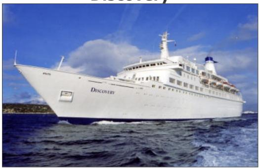
The M.V."Discovery" is a 20,216 tons single ship operation catering for the exotic destination market. The vessel was built in 1972 in Germany as the "Island Venture" but spent the 1974 to 2001 period as the "Island Princess" of Princess Cruises. Between 2002-03 she underwent an extensive rebuild returning to service in mid 2004. She carries 650 passengers when cruising and has a crew of 305.
